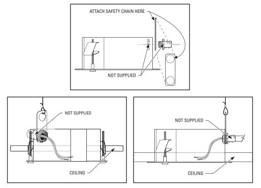
Figure 4. Installing the Back Box
